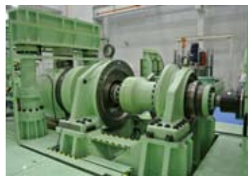
Evaluation test equipment for evaluating large size bearing
