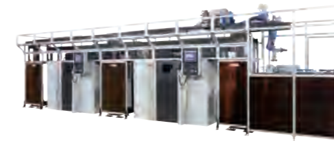
Grinding system integrating in-line measurement that maintains the production of quality products
