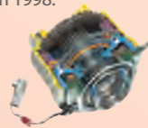
4WD electronic intelligent torque-controlled coupling (ITCC)
