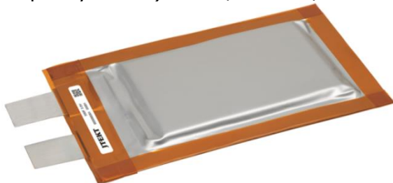
An example of a capacitor (500F cell single-part product)
