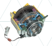
4WD electronic intelligent torque-controlled coupling (ITCC)
