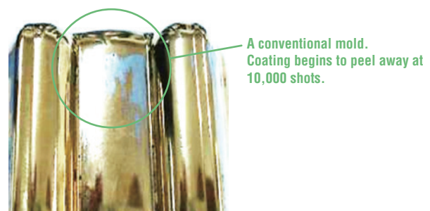
▶ Figure-02 Extended mold life by applying a new coating
