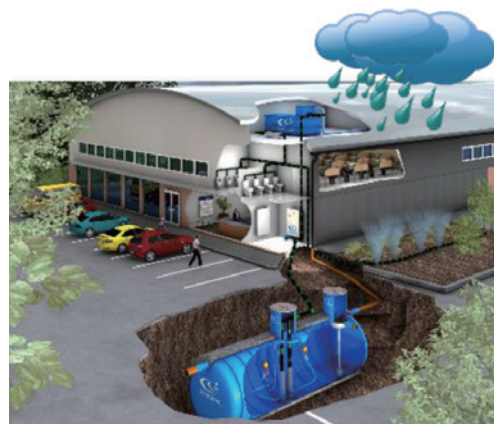
Rainwater storage system (JAUk, U.K.)
