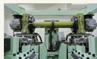
Testing machine for bearings made for high-speed railroad vehicles
