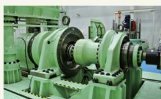
Evaluation testing machine for ultra-large bearings
