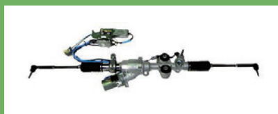
Newly developed rack coaxial type EPS
