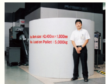
In front of a workpiece model showing the machine's maximum machining range and load
