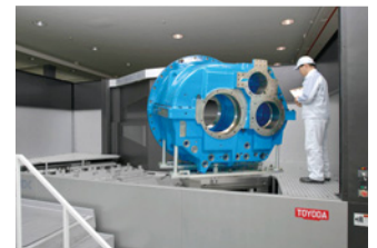
Inspecting the machining finish of a windmill power generator gearbox on a 1,250mm square pallet. This machine can machine large parts with the widest machining range, fastest feed speed, and strongest cutting performance in its class.
