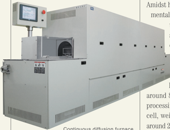
Continuous diffusion furnace
