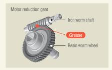
In 2012, JTEKT developed grease for the EPS reduction gear that achieves both a superior low friction characteristic and high compatibility with resin. This grease greatly improves the performance and reliability of resin wheels by increasing service life by roughly 1.8 times and raising reduction gear efficiency by 16.5 percent.
