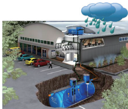
Rainwater storage system (JAUk, U.K.)
