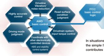
Using wheel speed signal, throttle position signal, etc. that come as standard equipment in the vehicle, ITCC basic control logic compatible with traction performance and tight corner binding avoidance is developed
