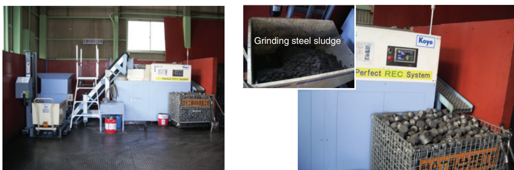
(Left: a full view of machine, Right: Value Pack produced by the machine)
