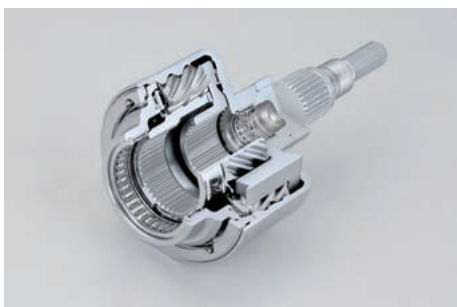
Fig. 22 Appearance of developed planetary gear type torque-sensing LSD (Vehicle B type)
