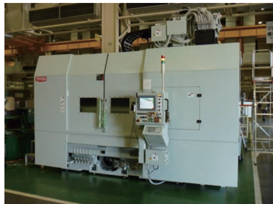
Fig. 1 VGX-100 super-large vertical grinding machine
