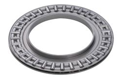
In recent years, the use of low viscosity lubrication has become widespread for improved fuel efficiency in automobiles. While thrust needle roller bearings are known for high load carrying capacity, their friction loss is large due to a structure with high sliding contact. Also, there have been issues with wear occurring easily on both sliding and rolling contact areas under low viscosity lubrication conditions.
