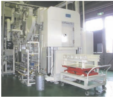
Vacuum Carburizing Furnace
