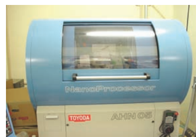
Fig. 7 Newly-developed fluctuation-free ultra-precision aspherical grinding machine
