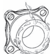
Fig. 5-a Image of water influx onto the end face of the outer ring
