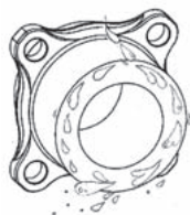
Fig. 5-b Image of water retention on the end face of the outer ring during axle rotation
