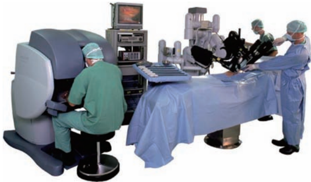
Fig. 1 DA VINCI surgery “robot” (or telemanipulator) from Intuitive Surgery inc
