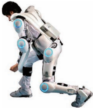
Fig. 4 “Robot Suit” human assist device HAL from Cyberdyne, Japan
