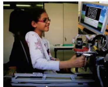
Fig. 2 Two degree-of-freedom (d.o.f) hand rehabilitation device designed at EPFL Robotic Systems Lab for hemiplegic children
