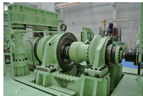
Fig. 4 Actual size bearing evaluation testing machine
