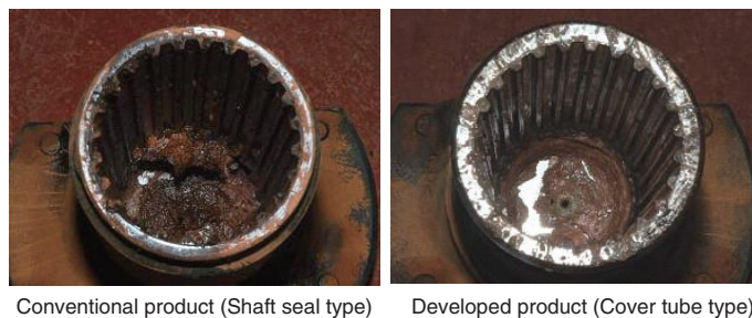
Conventional product (Shaft seal type) Developed product (Cover tube type)
