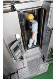
Main operation panel and easily accessible operation door
