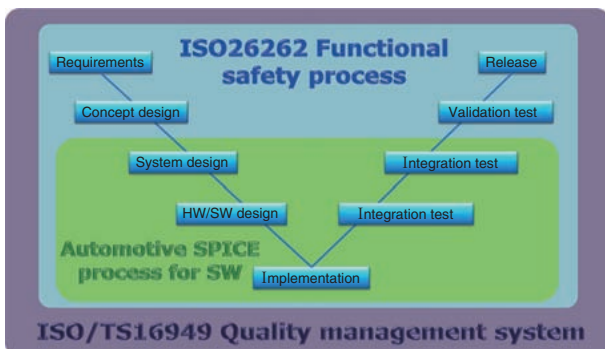
Fig. 7 V-model of functional safety
