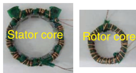
Fig. 5 VR resolver used for real machine examination
