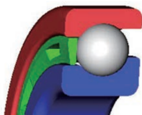
Fig. 12 High axial load-compatible ball bearing
