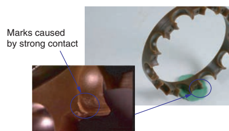
Fig. 2 State of snap cage after high-speed test
