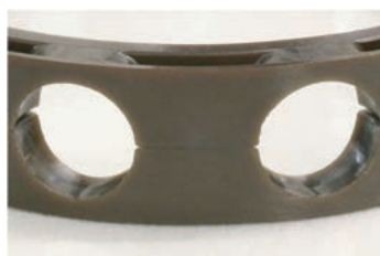
Fig. 13 Appearance after high-load durability test
