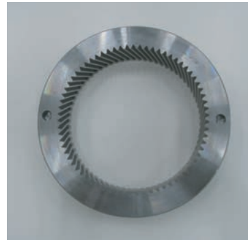
Fig. 9 Example of machining ring gear
