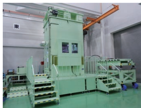
Fig. 6 Bearing test rig for steelmaking equipment 6)
