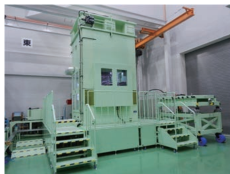
Fig. 13 Bearing test rig for steelmaking equipment
