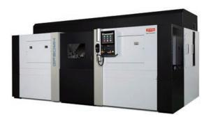
Being equipped with two wheelheads, the GF50Mi-70T grinder can perform simultaneous cutting of both a crankshaft pin and journal with two wheels. This report introduces our newly developed product, which have improved productivity, flexibility and reliability of the grinder to meet the demands for higher labor productivity and small lot production of multiple models in automobile engine manufacturing.
