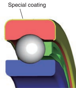
Fig. 8 Ball bearing coated with special coating for preventing electric pitting
