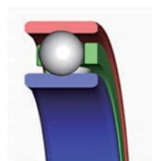
Fig. 27 Thin section ball bearing for wave reduction gear
