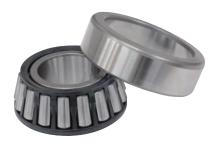
Tapered roller bearings are used mainly in the differentials and transmissions of automobiles. JTEKT developed an ultra-low friction torque tapered roller bearing with low friction torque, improved anti-seizure, and extended bearing life in contaminated oil compared with the conventional tapered roller bearing. Volume production of this bearing for transmissions of Japanese automobile manufacturers is planned. This report introduces the features.
