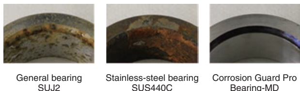
Fig. 12 CASS test results
