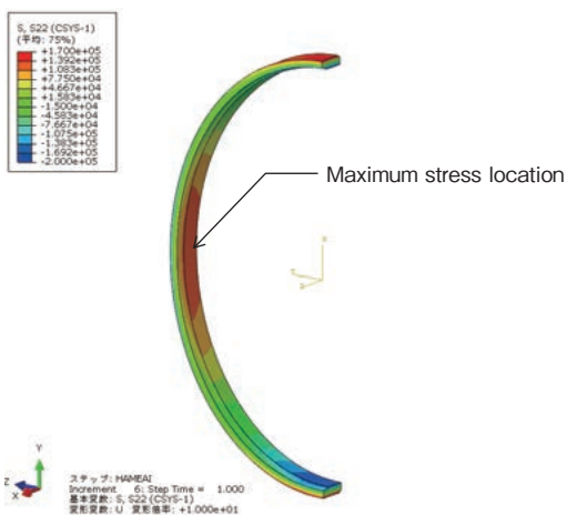
Fig. 4 Analysis example of outer ring strength (typical example)
