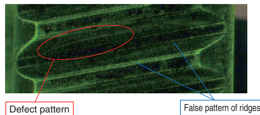
Fig. 2 False indication on rack teeth ridgeline
