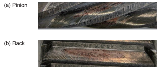
Fig. 11 Tooth surface after endurance test
