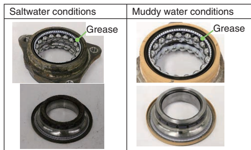
Hub unit assembly test (water injection conditions)
