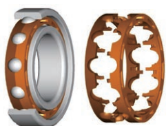
Fig. 2-1 Two-piece cage shape
