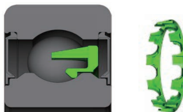
Fig. 3-1 Newly developed bearing shape (Cage with new shape)
