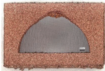
Fig. 10 Water pipe collapse
