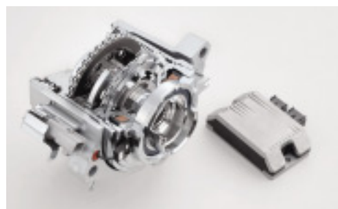
An ITCC and a control unit
