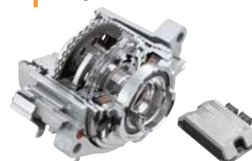
Electronically controlled four-wheel drive coupling (ITCC)
