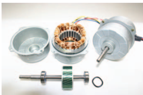
図2 エアコンモータと軸受の外観 Appearances of air conditioner motor and bearing
