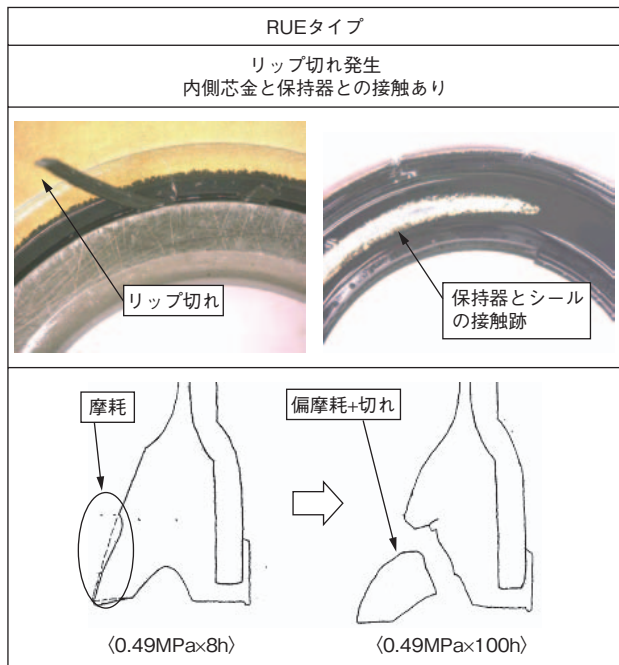
図4 過大油圧でのRUEタイプの破損形態 Failure mode of RUE type seal under excess oil pressure
