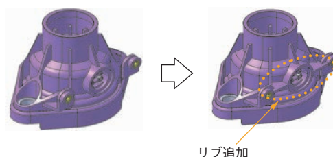
図5 リブ追加例 Case example of rib addition
