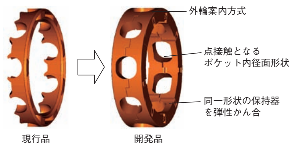
図9 開発保持器形状 Form of developed cage
