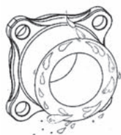
図 5-b 軸回転中の外輪端面の水滞留イメージ Image of water retention on the end face of the outer ring during axle rotation
