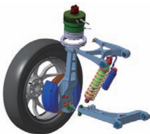
図7 研究用車両 SpeedE の車輪独立転舵の前軸 Wheel individual steerable front axle of the research vehicle SpeedE
