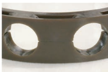
図13 高負荷耐久試験後の外観 Appearance after high-load durability test
